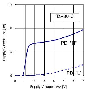
Figure 1. Supply Current vs Supply Voltage
