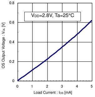
Figure 5. OS Output Voltage vs Load Current
