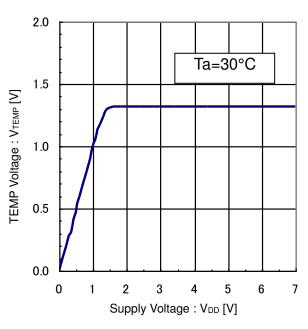
Figure 2. TEMP Voltage vs Supply Voltage
