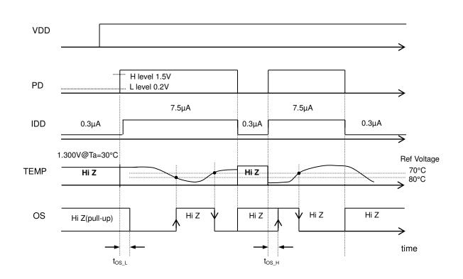
BDJ0801HFV operation starts after PD "H" Input. Please refer to the OS terminal signal table below for the wait time after PD "H" Input.
