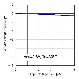
Figure 4. TEMP Voltage vs Output Current
