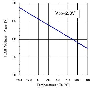
Figure 3. TEMP Voltage vs Temperature
